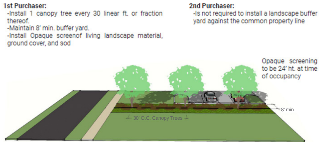
Figure 6.2: Abutting Property Requirements Against Purchaser/Lessee Properties
